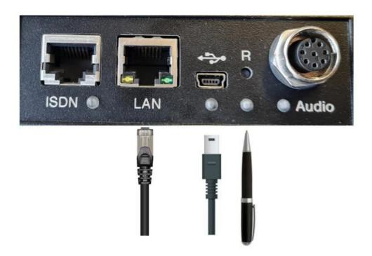
Press the reset button marked R **continuously**. The best way to do this is with a pointed object, such as a ballpoint pen or paper clip. To supply the ULE with power via PoE and to initiate the start-up process, the network cable must be plugged into the LAN socket. Wait until the ULE614 boots up in the boot kernel (you can see this under "Baugruppeninfo" (Module info)). This can usually take up to 20 seconds.
